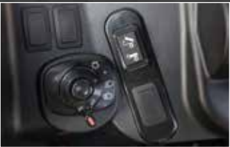
Electric hydraulic bed lift kit (left: dump switch / right: lift cylinder)
